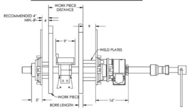
34" PLUS WORKPIECE DISTANCE = MINIMUM BAR LENGTH
